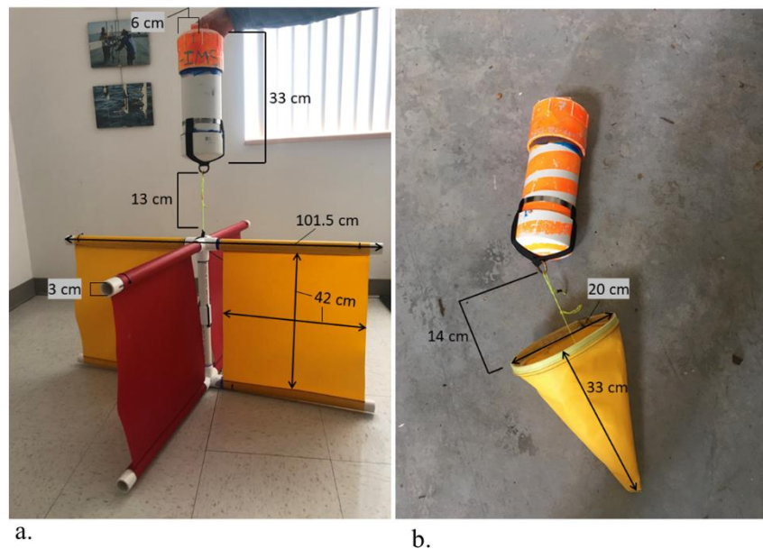
Figure 1. a. Davis Style Drifter with dimensions b. Cone Style Drifter with dimensions
