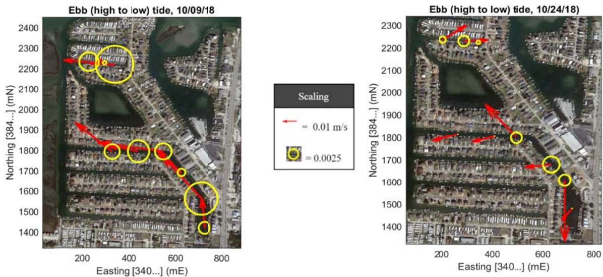
Figure 2.4. Velocity and direction from drifters released at ebb tide. Each point represents the averaged values of the drifters released at that point. Yellow circles represent the standard deviation of each group of drifters.
