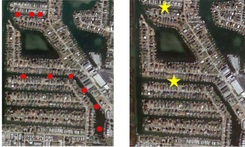
Figure 2.1: Short and long canal, with a) red circles indicating drifter release drop points in the canals and b) yellow stars indicating locations of current profilers.
