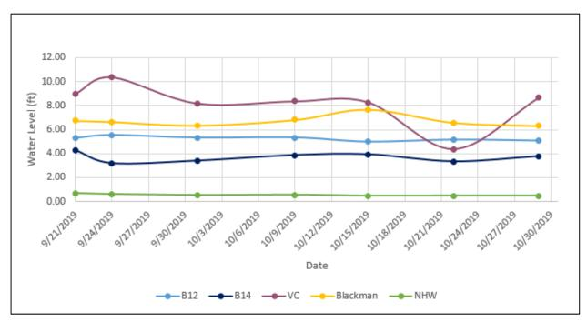
**Figure 7. Water Table Elevation Time Series.** Water table elevation (ft) for each groundwater sampling well in the Gallery Row subwatershed over the course of the study period from September 21, 2019 to October 29, 2019. Each well is represented by a different colored line.
