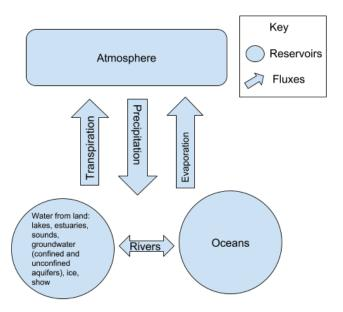
**Figure 1**: Basic diagram of the hydrological cycle, depicting global reservoirs and the fluxes of water that move liquid and gaseous forms of water between them (adapted from Chahine, 1992).
