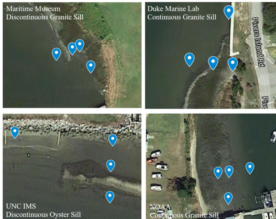
Figure 1. Maps showing locations of pressure sensors at each of the four living shorelines. Each site has one sensor in front of the sill, one directly behind the sill, one along the shore in line with the two previously mentioned sensors, and one sensor along the shore that is not behind the sill.
