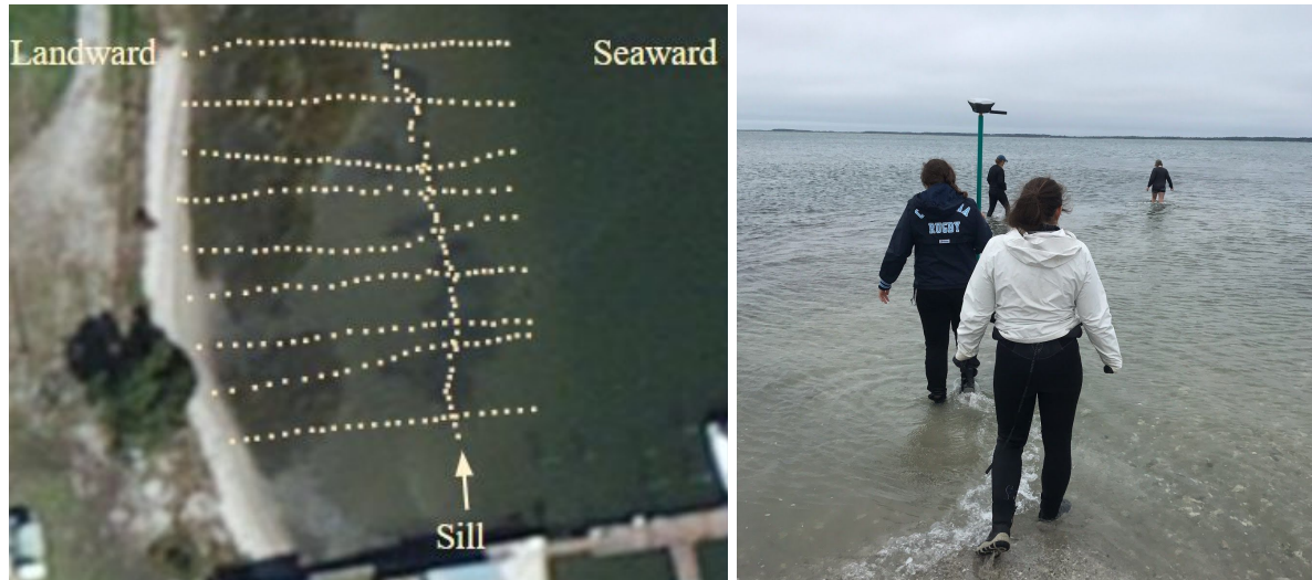
Figure 4. (Left) Continuous oyster sill transects and points, at which latitude, longitude, and elevation data taken using the EMLID. (Right) Photo of team members performing elevation surveys.
