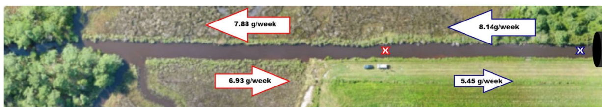
Figure 3. TIMS sampler deployment location, the channel (red) and pipe outfall (blue) marked by the x. The bi-directional samples measured sediment amounts from the flood direction (flow from left to right) and the ebb direction (from right to left).
