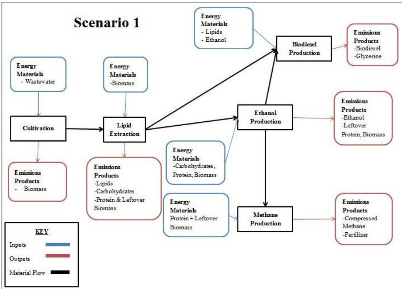
**Fig. 2:** Scenario 1 process diagram. Scenarios 2 and 3 follow similar processes, but Scenario 2 excludes "Ethanol Production", and Scenario 3 excludes "Lipid Extraction," "Biodiesel Production," and "Ethanol Production."
